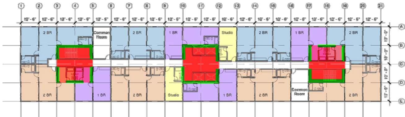
Figure 4: Typical Building Floor Plan (Core areas are highlighted in red, core walls are highlighted in green)
